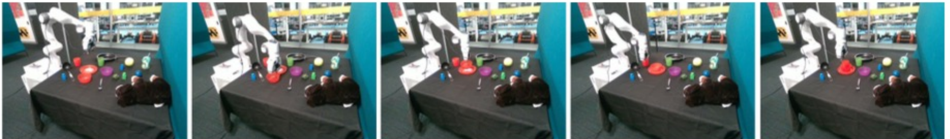
Fig. 3: Sub-tasks decomposition of a Place the bowl on the plate and the cup in the bowl matching the color sequence.
